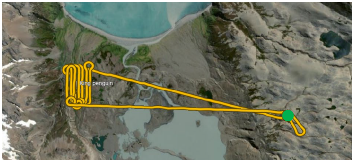
Figure 2. The flight path of the king penguin colony survey at Fortuna Bay. The take-off area (green dot) is located within the KEP field operational area, whereas the penguin colony is not. BVLOS made the survey of this site possible.
